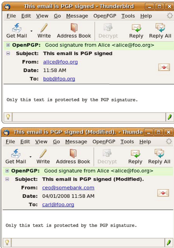
Fig. 1. A signed PGP mail in Thunderbird 2.0 with PGP plug-in Enigmail. The original message (top) is sent from alice@foo.org to bob@foo.org . In the modified message (bottom), the From field is changed to ceo@somebank.com , the fields To , Date , and Subject are also modified; however, the signature is still treated as valid in Thunderbird.
